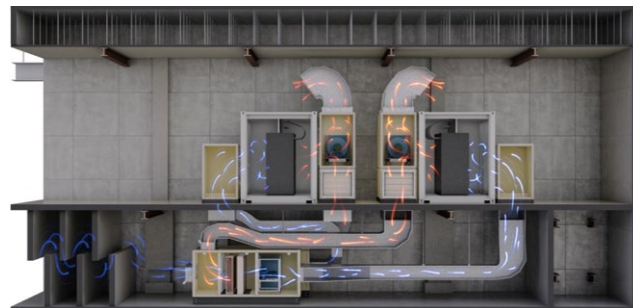
Four-season outdoor air conditioning system in Busan Data Center
